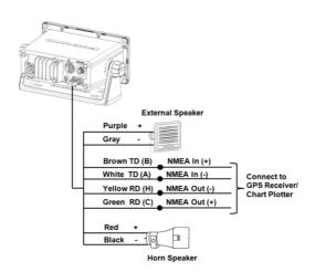
The NMEA 0183 wire should be connected to a compatible NEMA 0183 device as shown in the table below:
